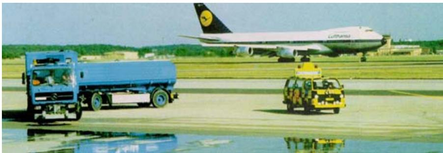
The various types of deployment vehicles can be equipped with a continuous adjustable hydraulic low-speed drive, marking it possible to proceed steadily even at extremely low speeds - eg, during runway marking work.
