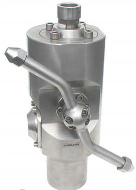
Type XXL 1500-2 56 mm lever arm, 2 nozzles max. 1500 bar / 500 l/min. Min. Tank access: 500 mm
