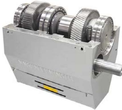
The integral speed reducer with twin helical gears arranged in a herringbone configuration ensures smooth running and even power transmission without axially loading the bearings.
