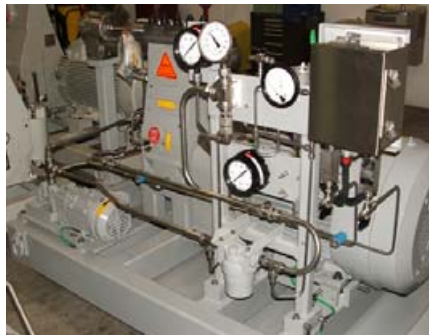
HDP 72 unit for methanol duty Op. pressure 12,000 psi – 830 bar Flow rate 6 gpm – 24 l/min
